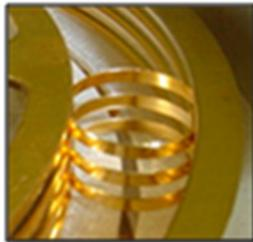
Each circuit is separated by insulators in the axial and radial directions. Rotor and stator are precisely aligned with bearings to ensure proper rotation for long life. The rolling electrical interface is made shock and vibration tolerant due to the compression otherwise known as pre-load of the flexure between the rotor and stator grooves. Seals are added as necessary for the specific application environment.
